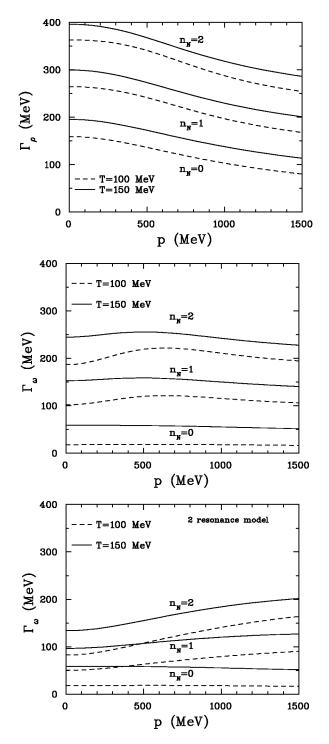
FIG. 6. The vector meson widths as a function of momentum p. Results are shown for nucleon densities of 0,  $n_0$ , and  $2n_0$  (where equilibrium nuclear matter density  $n_0 = 0.16 \text{ fm}^{-3}$ ) and temperatures of 100 and 150 MeV. For the  $\omega$  meson results are given for the multiresonance and the two-resonance models.
